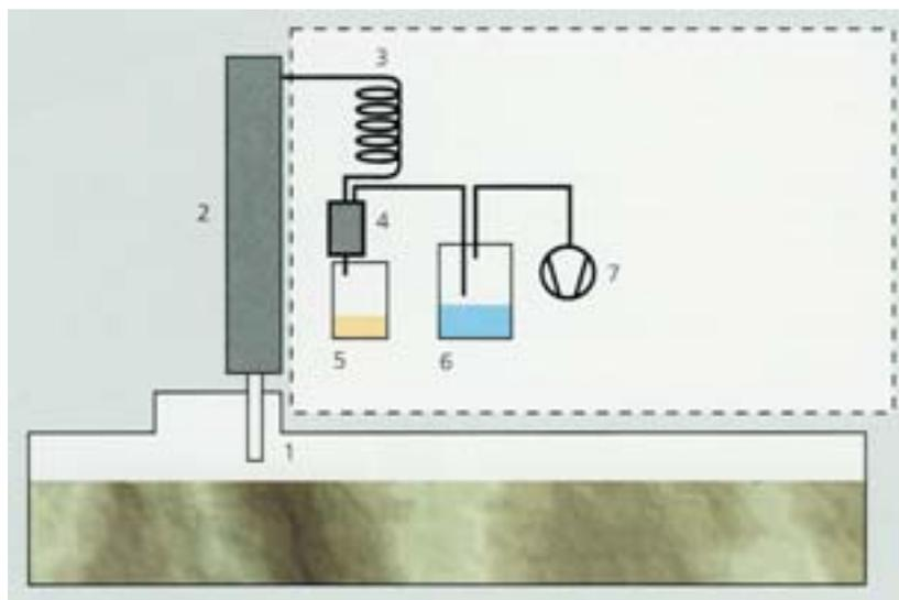
Figure 5: Apparatus for collecting condensate from bitumen. The fume/aerosol mixture is collected in a cooler (4) and a vessel (5) from the heated (180 °C, 356 °F) bitumen tank using a heated tube (2) and a stainless steel coil (3). A further vessel (6) is used as a waterfall and protects the pump (7). It should be noted that this temperature is on the high side of those typical of rolled asphalt applications.
