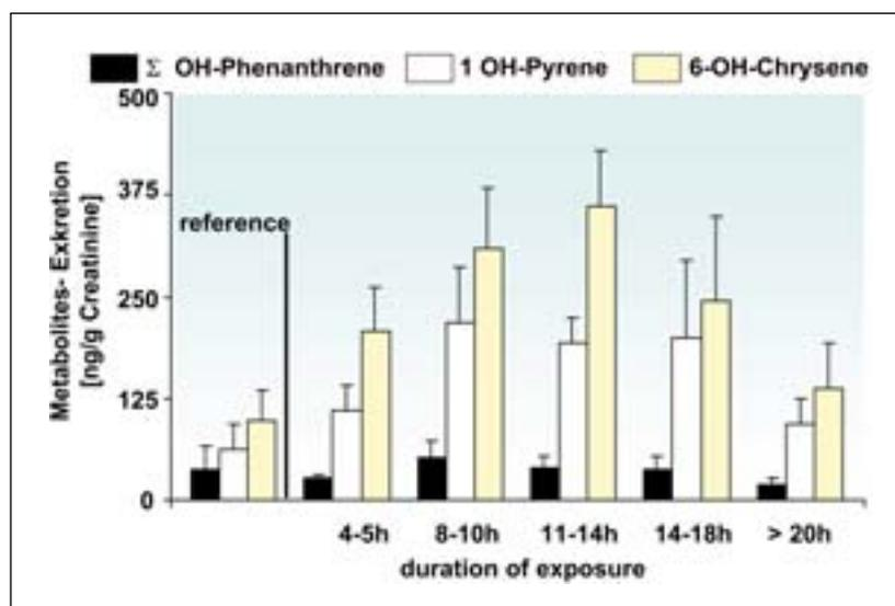
Figure 6: Concentration of three PAH metabolites from 10 test persons wearing breathing equipment before, during and after exposure to vapour and aerosols of bitumen of 20 mg/m<sup>3</sup>
