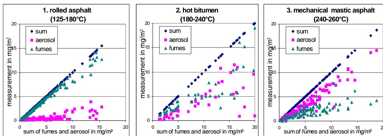
**Figure 1:** Comparison of the proportions of fumes and aerosol concentrations from hot bitumen. 1. Working with rolled asphalt in road paving. 2. Working with hot bitumen in pouring process. 3. Mechanical working with mastic asphalt in road paving. The diagram shows only values up to 20 mg/m<sup>3</sup> in the cited working temperature range.
