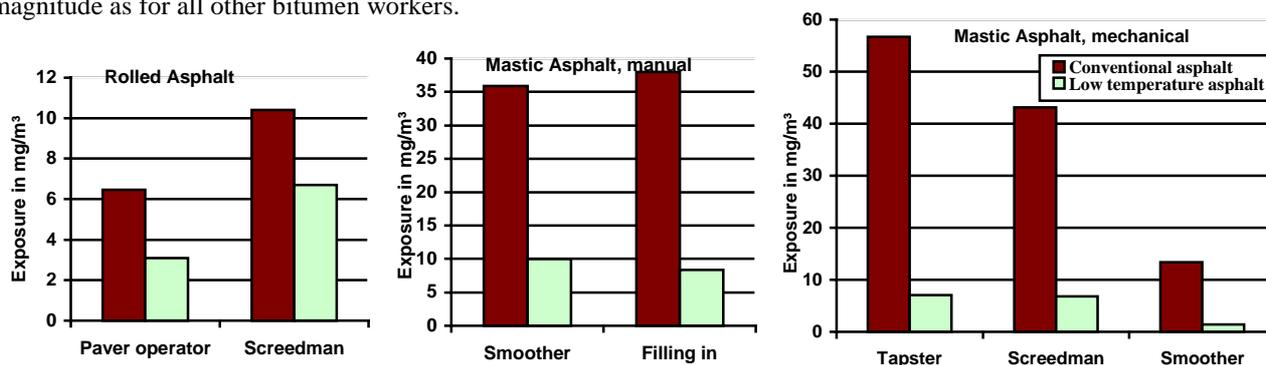
**Figure 3:** Exposure to fumes and aerosols from bitumen by laying normal and low temperature asphalt
