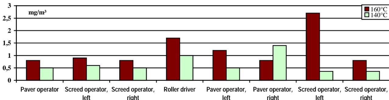
**Figure 4:** Comparison of exposure to fumes and aerosols from bitumen by laying normal and low temperature asphalt at a construction site in France
