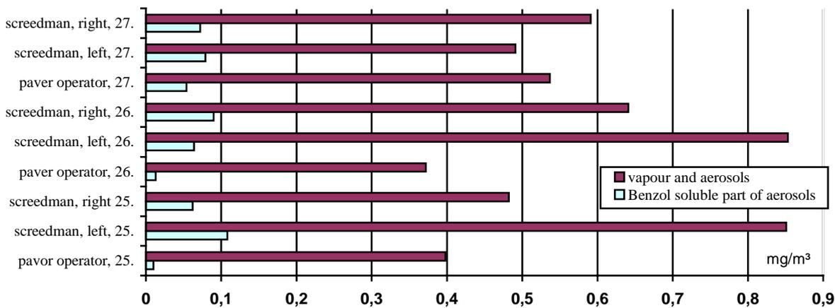
**Figure 2:** Measurements comparing the United States (benzol soluble part of aerosols) and the German procedure (fumes and aerosols) (asphalt temperature 160°C; Shell, 1999)
